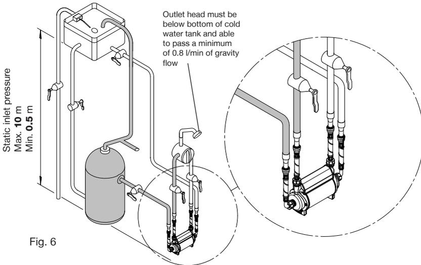
2.25 **The cold water supply: Must be a DEDICATED AIR FREE** supply via a tank connector, and must be positioned at a slightly lower level (25 mm minimum) than the feed pipe to the hot water cylinder.
